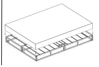
**3.** Place the Bundled slat sections (D) in the middle on each side snapping each slat end into the plastic seat.
