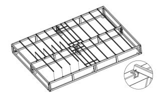
**2.** Align the middle support with the metal flaps pointing away from the hinge section and attach using the longest bolt thru the hinge section, repeat the same on the opposite side. Align each corner with the vertical supports and attach using 10 bolts, 1 thru each support, the other by the leg plate. Tighten all nuts with the **enclosed wrench**.
