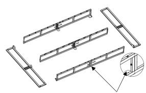
Thru the unfolded hinge, insert and tighten 1 Screw and nut
