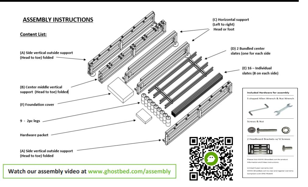
**1.** Unfold the side vertical outside supports (A) placing them approx. 4 feet apart **with the hinges facing inward**. Unfold and place the center middle vertical support (B) in between the 2 supports.
